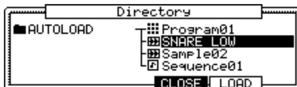
The folder selected in the folder field is displayed in the left of the directory list, and the files selected in the File field are displayed in the right of the list. In the picture above, the SNARE LOW file in the AUTOLOAD folder is selected. Each file has an icon according to their types.
