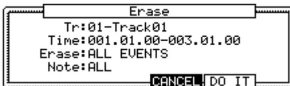
The Tr field displays the number and the name of the selected track. To delete all the events of the track, select "Tr:00- ALL TRACKS" by turning the DATA wheel to the left.
