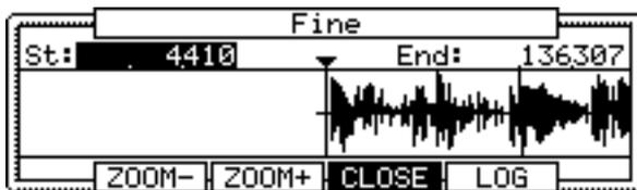
In the Fine windows, the waveform display varies depending on the location of the cursor. When you select the St (Start) field with the cursor, it displays the start point in the center of the window. When you select the end field, it displays the end point in the center.
